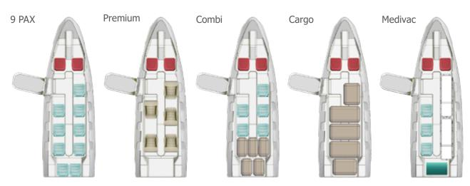
TE RANGI offers versatile configurations to meet a wide range of operational needs, making it an adaptable and cost-effective solution for various sectors. The aircraft can be configured for passenger transport, air freight, or special missions like medical evacuation and long-range air surveillance. What sets TE RANGI apart is its flexibility. Operators can easily adjust the aircraft's configuration
